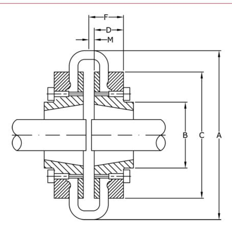
$\begin{array}{lll} A & = 405 \\ B & = 197 \\ C & = 347 \\ D & = 77.4 \\ F & = 92.4 \\ For taper bush = 4030 \\ M & = 15.0 \end{array}$
